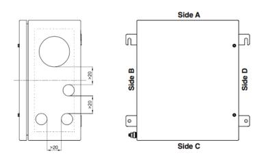
All enclosures can be equipped with accessories of your choice and mounted on special rails attached to the internal mounting frames of the housing. The terminal blocks can be arranged in different ways, according to the customer's specifications and always within the limits allowed by the certificate. The options are vertical, horizontal, on a number of rows or on different levels using appropriate spacers.
