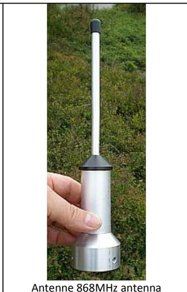
Antenne 868MHz antenna
